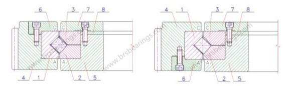
2. On the standard platform, install the crossed tapered roller bearing onto the shaft or into the bearing housing. Install the 6&7 flanges in sequence as shown in the figure above, lock the screws in diagonally opposite sequence follow the order as shown in below diagram when tightening bolts. Do not tighten bolts randomly. Then use a thickness gauge to check whether the flanges are properly installed.
